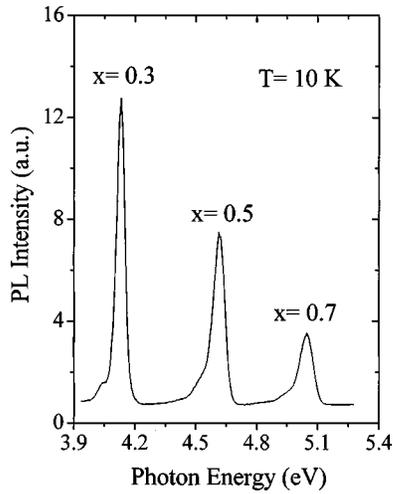
FIG. 1. Photoluminescence spectra in  $\text{Al}_x\text{Ga}_{1-x}\text{N}$  alloys measured at 10 K for Al concentrations  $x=0.3$ , 0.5, and 0.7.
