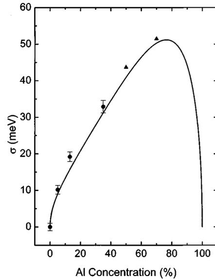
FIG. 2. Variation of excitonic linewidth ( $\sigma$ ) as a function of Al concentration: theoretical calculation according Eqs. (1 and 2) (solid line), determined from the line shape analysis of our PL spectra measured at 10 K (triangles). Circles represent our earlier data.
